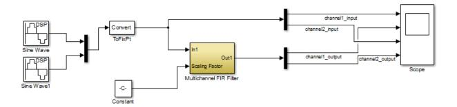
The model includes a two-channel sinusoidal signal source feeding a filter subsystem targeted for HDL code generation.
