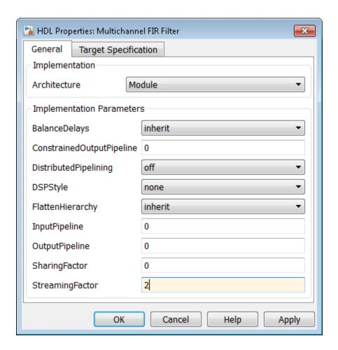
Set the **StreamingFactor** to 2, because this design is a two-channel system.
