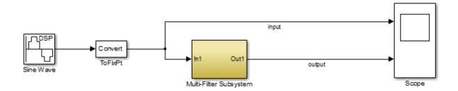
The model includes a sinusoidal signal source feeding a filter subsystem targeted for HDL code generation.
