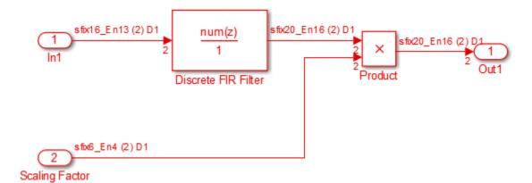
The subsystem contains a **Discrete FIR Filter** and a constant multiplier. The multiplier is included to show the optimizations operating over all eligible logic in a subsystem.
